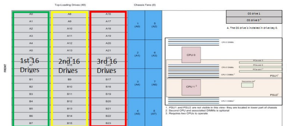
Figure 2. The following highlights illustrate the slots to be populated in order from left to right as disks are added for the three configurations noted in the above table.
